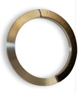
They consist of a metal sealing core (with or without a guide ring) with concentric serrations on both sealing surfaces and faced with a soft material such as flexible graphite, ePTFE, or a Lamons high-temperature gasket (HTG) configuration. Kammpro is the preferred design when improved performance at lower seating stresses is needed, and it can be manufactured in different core materials and shapes with extreme accuracy. It can also be custom engineered to fit various applications.
