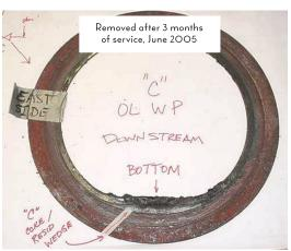
Pictures revealed petroleum coke buildup at the bottom of the gasket. As the graphite oxidized, the coke would fill in the voids causing the gasket to leak, acknowledging the need for a more reliable sealing solution.
